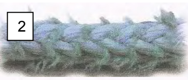
> Image 2 Rope displaying 25% reduction from abrasion
