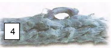
> Image 4 Strand reduced by 25% abrasion
