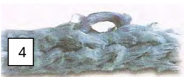
> Image 4 Strand reduced by 25% abrasion
