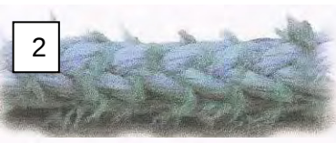
> Image 2 Rope displaying 25% reduction from abrasion
