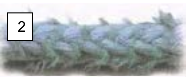
> Image 2 Rope displaying 25% reduction from abrasion
